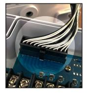
Connect the head to the base plate by first plugging in the connector. Push connector all the way so that the thumb latch is effective.
