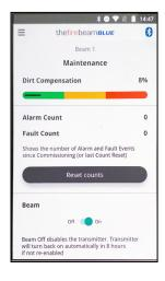
Here we can see if any compensation has been made for dust build up and whether any alarm or faults have occurred. You can also turn the beam off here
