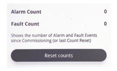
Here we can see how many times the beam has gone into fire or fault since the beam was commissioned or since the event log was last cleared including testing. You can also reset the counts here
